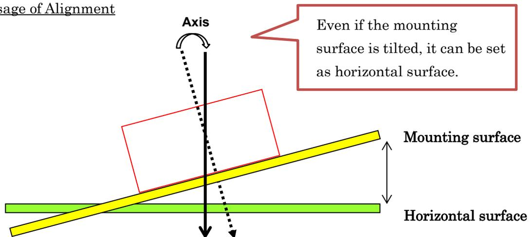
By sending RALN command (Alignment compensation reset), it is possible to return to the initial setting.
