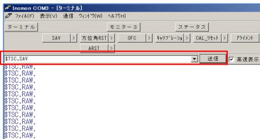
Request for RAW data output at your desirable output cycle. Enter the SAV command, and confirm the ACK response.
