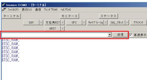
From the next startup, IMU outputs the data at the same cycle as when the SAV command is executed.
