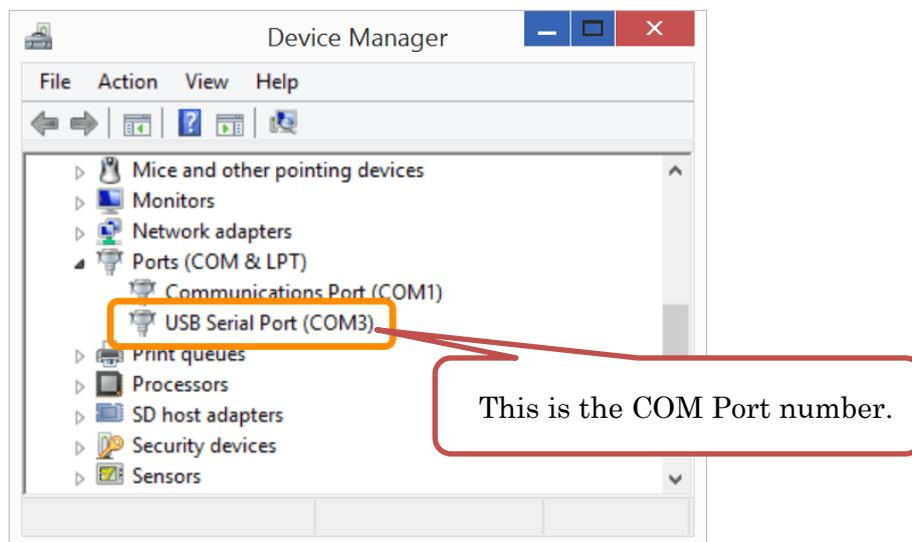
If COM port number is not displayed, you may need to install RS232C-USB driver. (If COM port number is displayed, RS232C-USB driver is already installed in your PC. You do not need to re-install the driver.)
