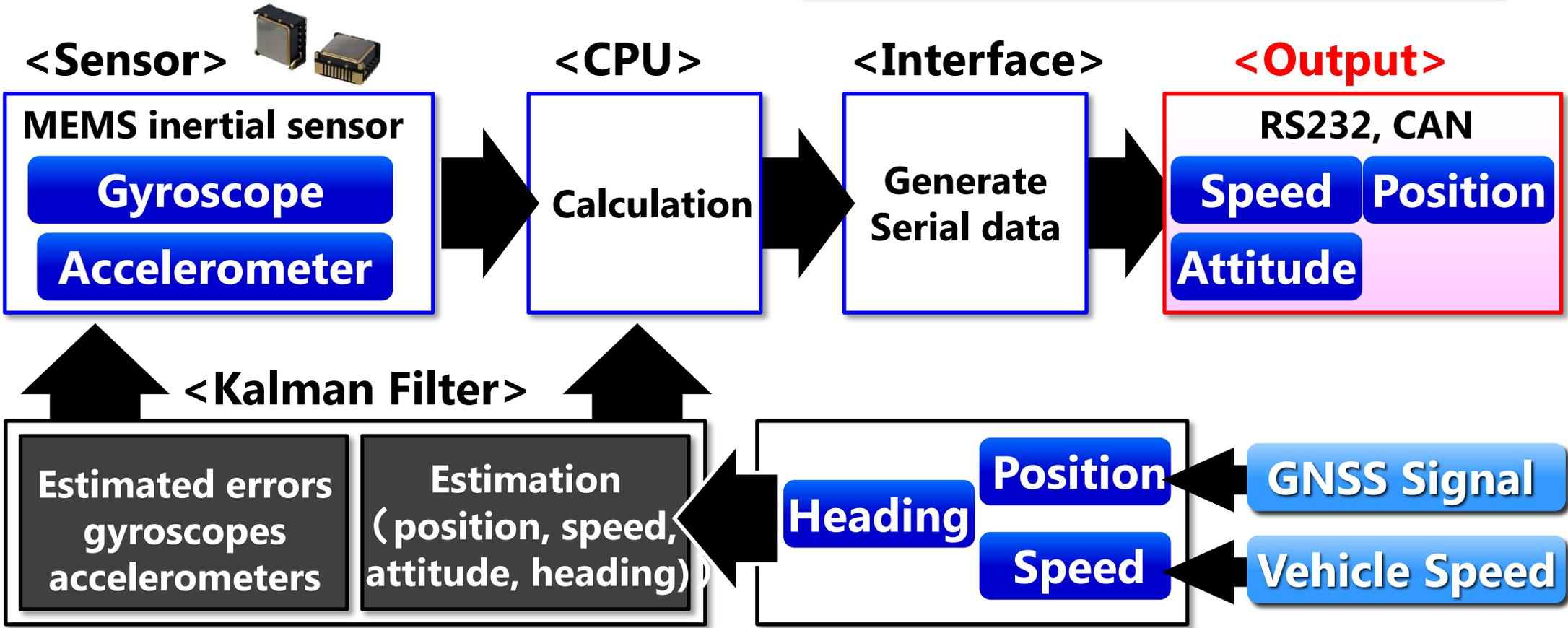
\* GNSS/INS/VS is performed by combining gyroscopes and accelerometers (INS data), external GNSS data and vehicle speed. Kalman filter estimates the errors of INS data.
